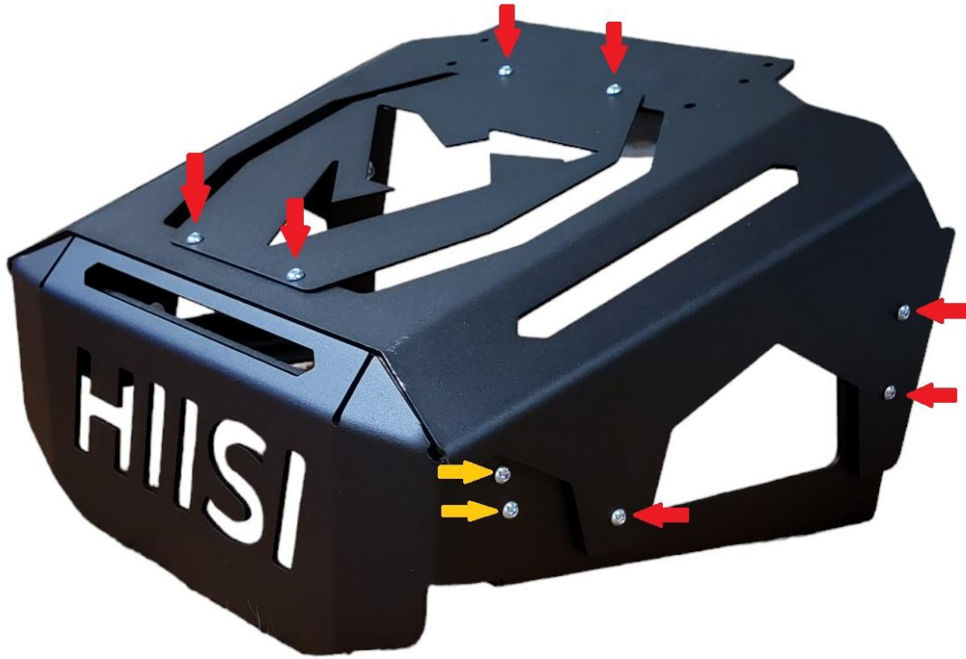
Assemble radiator cover. Red bolts 6x16mm and yellow bolts 6x20mm.
