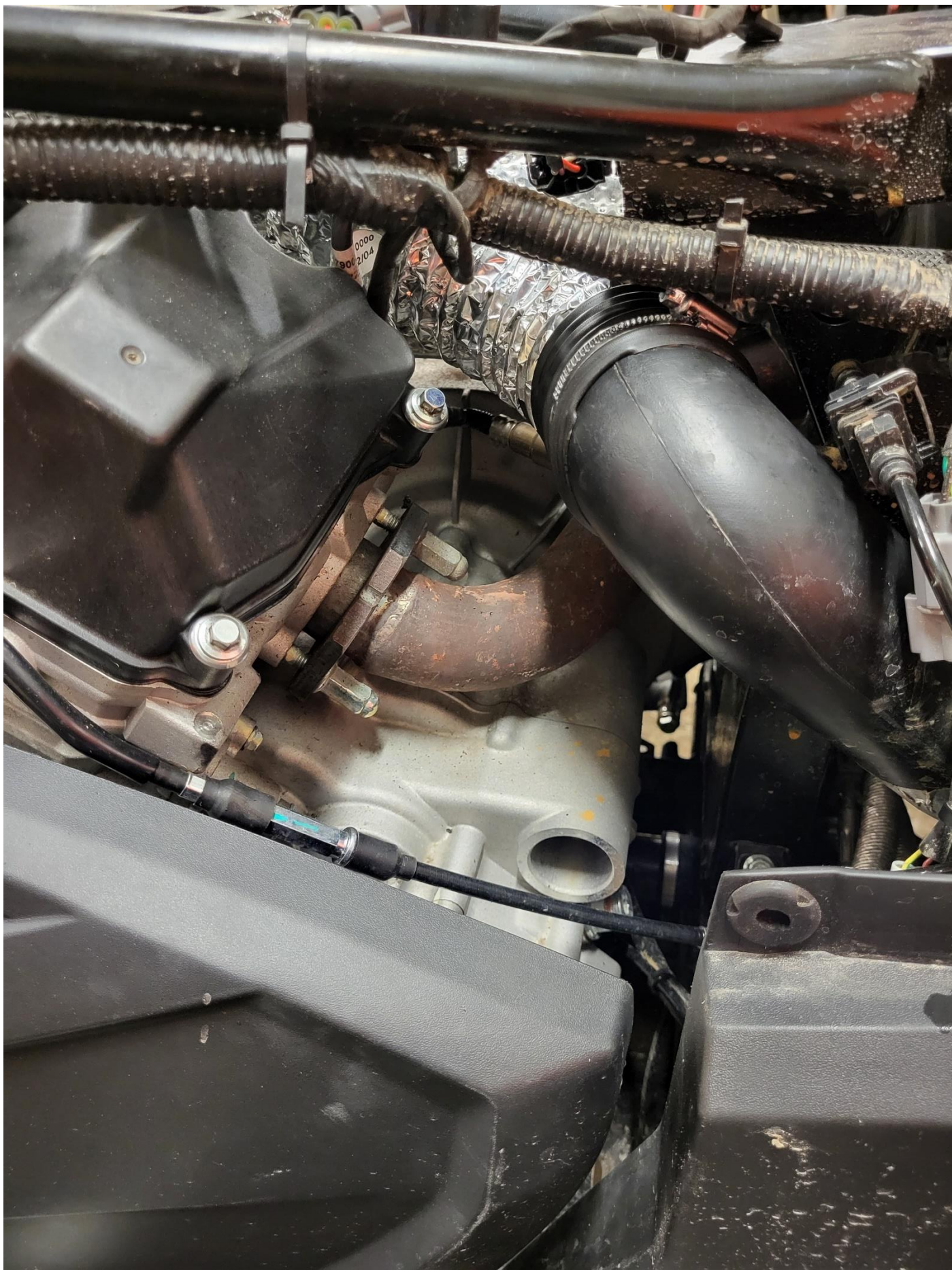
Connect hose to the CVT outlet pipe.
