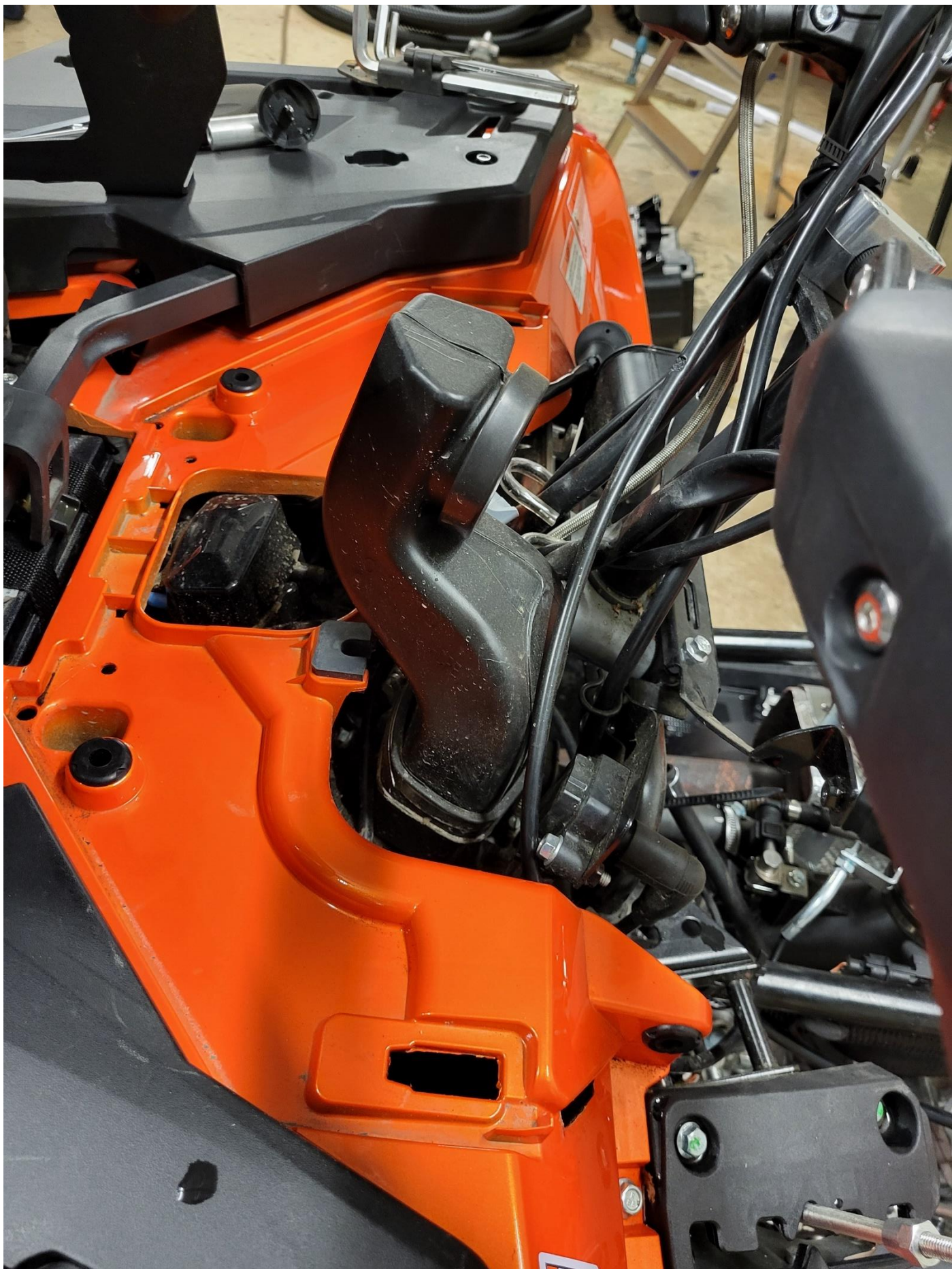
Remove engine intake pipe.
