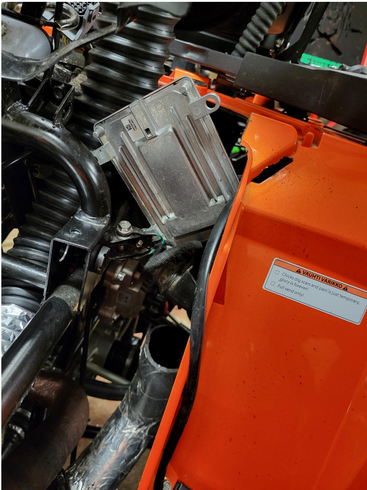
Install ECU as shown in picture.
